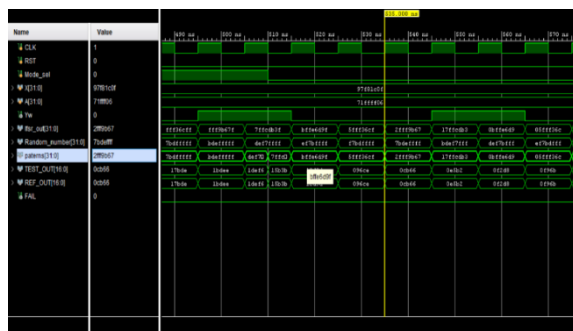
Fig 4.13: Simulated Waveform of the Proposed BIST Design
