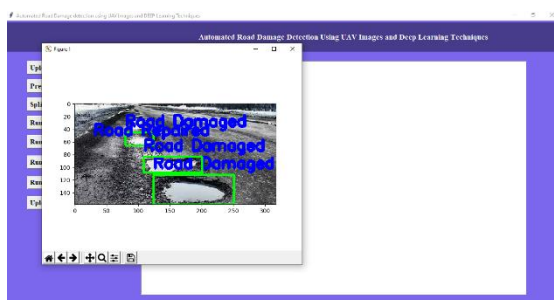
Figure 6: Road Damage Detection on Test UAV Images
