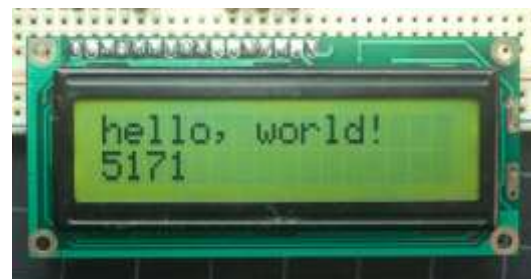
Output of the sketch on a 16x2 LCD
