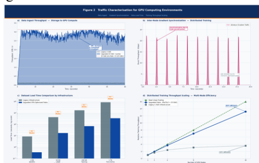
Figure 2 Traffic characterization for GPU computing environments. Panel (a) shows data ingest throughput from storage to GPU compute nodes comparing the legacy infrastructure to the upgraded fabric with jumbo frames. Panel (b) illustrates the bursty nature of inter-node gradient synchronization traffic, with concentrated pulses at iteration boundaries and idle periods during forward and backward passes. Panel (c) compares dataset load times across four representative dataset sizes on a logarithmic scale. Panel (d) presents distributed training throughput scaling with node count, comparing ideal linear scaling, the upgraded fabric with RoCEv2, and the legacy infrastructure.
