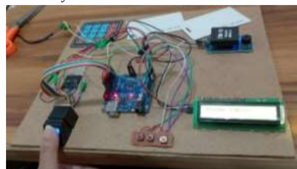
Fig 6.2: RFID-Based Transaction Tag Prototype with Arduino and LCD Display
